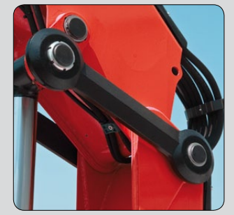
Forged double linkages on column and 2nd boom
