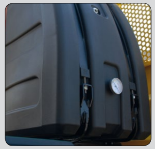
High volume oil tank made in sandwich-structured materials (PEX and PA6)
